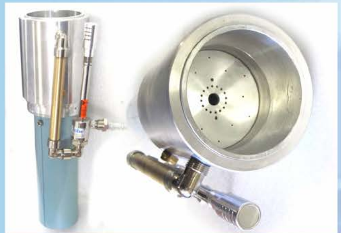
NEW EXTRA-COOLING SYSTEM with heat exchanger for prolonged flame spraying.
